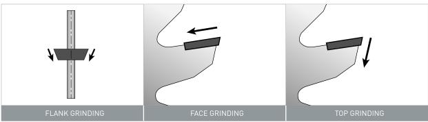
These steps can be carried out on a number of different machines, each needing its own grinding wheel geometry. With the unusually large range of Norton Winter grinding wheels available we offer the optimum tool for all machines and applications. The following table is colour coded to help you quickly and easily find the wheel you need for your saw grinding machine.
