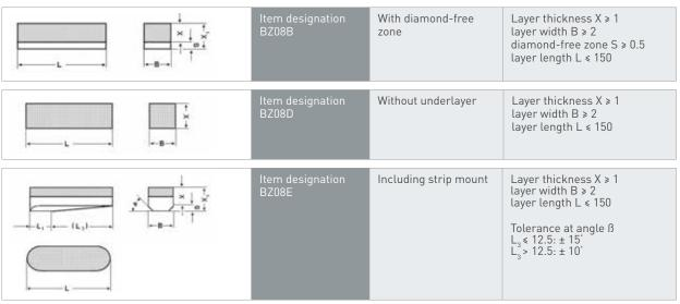
08B and 08D can only be used in conjunction with a strip mount. 08E is designed inclusive of strip mount for direct fitting.
