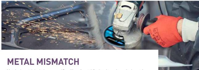
Metal mismatch includes removal/levelling of metal flash, tabs and panel mismatch around windows, door and boot openings plus excessive tack weld. Due to the aggressiveness plus high removal rates of the metal mismatch operation, it is imperative that the operator uses a continuous motion when levelling excessive material. This will eliminate the possibility of snagging the product while grinding and over-grinding the
