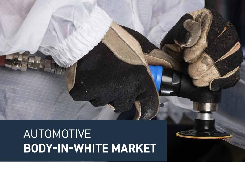
Body-in-white, which is the stage in the automobile manufacturing process in which a car body's frame has been joined together, before painting or another subassembly, sets the foundation for e-coat, primer, basecoat, and clearcoat. If manufacturers don't identify and remove defects in the body-in-white phase, the paint processes can accentuate imperfections or create paint defects.
