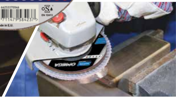
STOCK REMOVAL Flap Disc to remove heavy weld seams and excess material.
