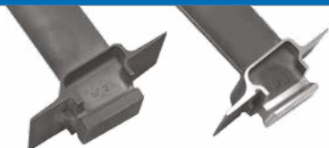
Fir tree before and after grinding
