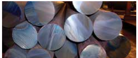
Dark cut (burns, blueing is visible)
