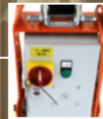
SELECTION OF THE WORKING ROTATION DIRECTION (CLOCK / COUNTERCLOCKWISE)
