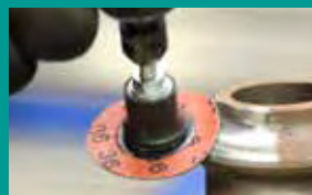
TIP Avoid gouging on contours by using a smaller size holder than the diameter of the discs, such as 38mm holder for 50mm.
