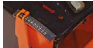
CUTTING DEPTH INDICATOR
