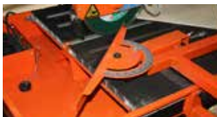
CUTTING GUIDE WITH ANGULAR SETTING
