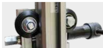
CARRIAGE GUIDING SYSTEM BY ROLLS.
