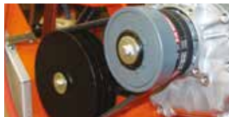
CENTRIFUGAL CLUTCH DEVICE (JUMBO P13 ONLY)
