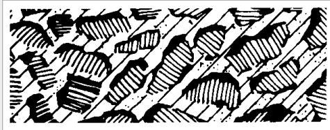
OPEN COAT (1/3 LESS GRAIN THAN CLOSED)
