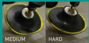
TIP Select a hard back-up pad for more aggressive applications.
