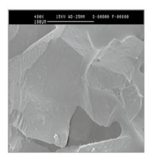
The characteristic formation of the bond bridges allows a high pore volume. On the left side a bond bridge is shown, which connects two grains.
