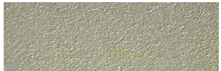
This is the same carbon surface after polishing with a Norton UltraLap Nanozyte M631 1-micron film disc. This scratch-free surface was obtained in one step.
