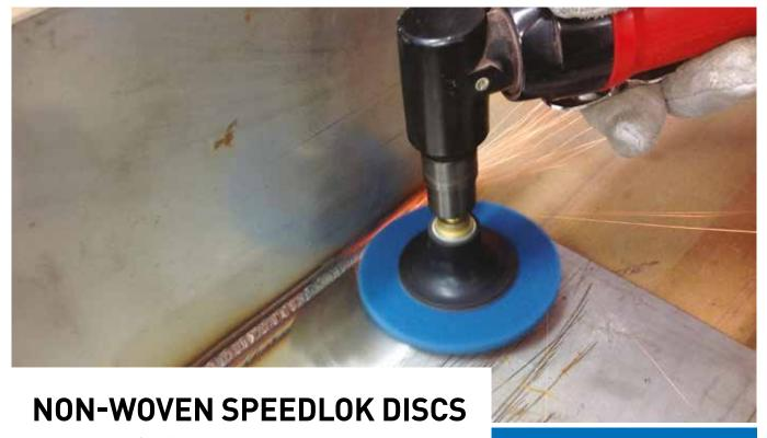
Norton non-woven SpeedLok quick-change discs are a combination of strong synthetic mesh and quality abrasives, bonded together by a smear-resistant adhesive. The open construction of the non-woven material enables aggressive cutting action and improved surface finish while maintaining its non-loading properties.
