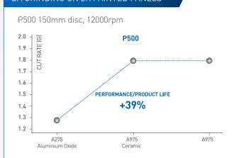
THE PERFORMANCE OF A975 IS SIGNIFICANTLY HIGHER THAN A275, AND PROVIDES EXCELLENT CONSISTENT CUT RATES. IDEAL FOR SCRATCH RESISTANT & CERAMIC CLEARCOAT.
