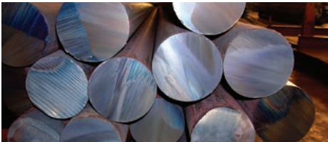
Dark cut (burns, blueing is visible)
