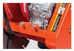
Quick Belt Tensioning Easy to change V belts for fast and accurate belt tensioning.
