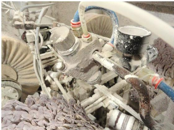
Figure 2. Conventional buffing is a messy, difficult-to-control process. Note the buffing compound splattered onto surrounding equipment and work space. Source: Norton | Saint-Gobain Abrasives
