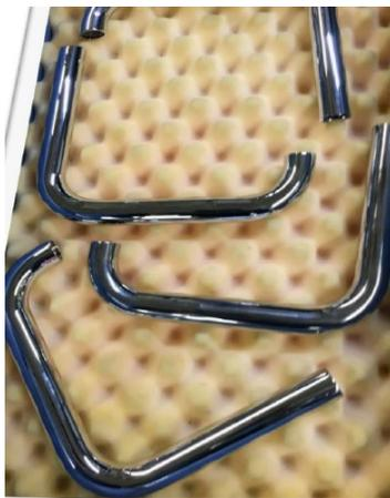
Figure 3. Nickel chrome plated FAB buffed parts showing a nearly unnoticeable amount of compound residue. Source: Norton | Saint-Gobain Abrasives
