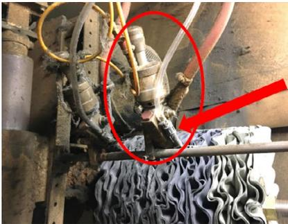
Figure 6. Liquid buffing compound (or water in select cases) is sprayed through nozzles (circled) and onto the buffing wheel to maintain coolness.
