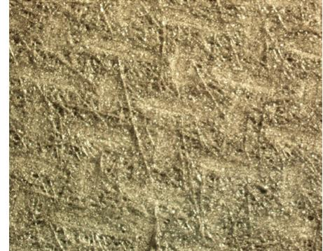
Figure 4. Magnified image of FAB surface showing abrasive slurry coating and non-woven nylon backing. Source: Norton | Saint-Gobain Abrasives
