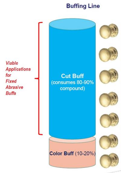
Figure 5. Norton FAB wheels are a viable replacement for conventional buffs in cut buffing, which consumes 90% of the compound. Source: Norton | Saint-Gobain Abrasives
