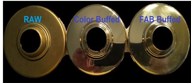
Figure 1. Raw, color buffed and FAB buffed brass rosette parts. Source: Norton | Saint-Gobain Abrasives
