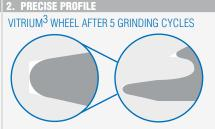
Superior grain-holding properties significantly improve wheel form and corner holding vs. other bond systems – reducing dressing time and dresser wear.
