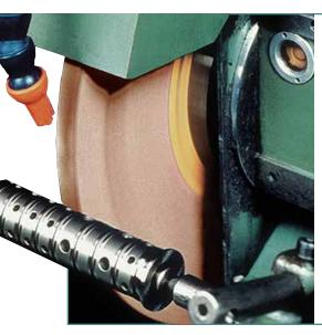
55A-VH blank stock wheels are competitively-priced, monocrystalline grain wheels specifically engineered for numerous carbon steel applications requiring moderate to heavy stock removal rates. They can be altered to your specific needs within two weeks of receipt of your order.
