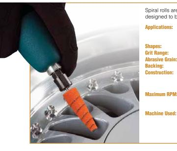
Spiral rolls are strips of abrasive cloth rolled and glued to form a solid shape that is designed to break down during use and reveal the next layer of abrasive.
