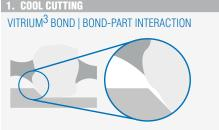
Improved holding power (using less bond-to-abrasive ratio) exposes a larger grain surface area, improving freer cut rate.
