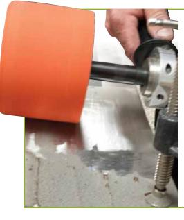
Portable belts are ideal for all your metal and woodworking applications. Choose 36 - 50 grits for rough/heavy-duty applications, 60 - 100 for intermediate, and 100 - 220 for finishing/polishing applications.
