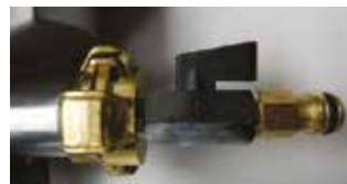
DUAL WATER-INLET AND DUST-COLLECTOR CONNECTOR
