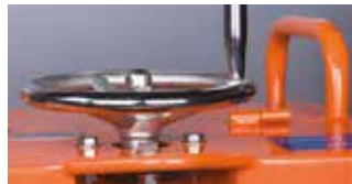
HANDWHEEL WITH ENDLESS SCREW DEPTH CONTROL SYSTEM
