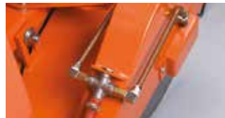
WATER ON BOTH SIDES OF THE BLADE
