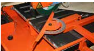
CUTTING GUIDE WITH ANGULAR SETTING
