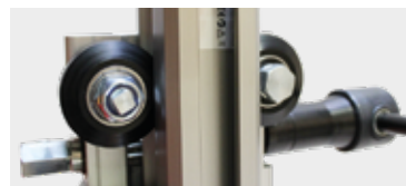
CARRIAGE GUIDING SYSTEM BY ROLLS.
