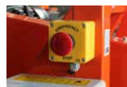
EMERGENCY PUSH BUTTON
