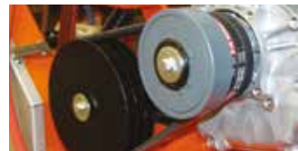
CENTRIFUGAL CLUTCH DEVICE (JUMBO P13 ONLY)
