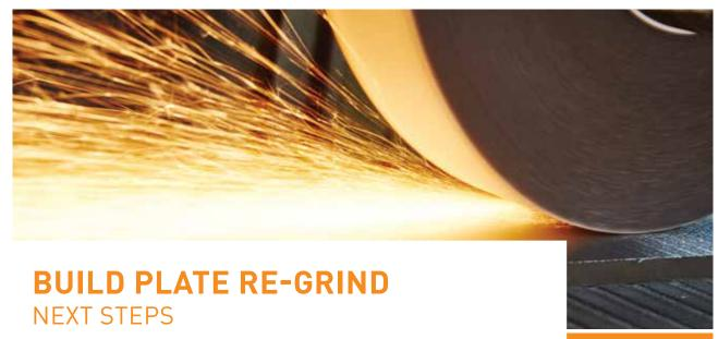
After the part has been cut and removed from the build plate, the plate must be prepared for reuse. Rotary or reciprocating surface grinding can be used to re-establish the required roughness, flatness, and parallelism of metal build plates. Norton surface grinding wheels using ceramic alumina abrasive grain are recommended to achieve a consistent surface finish with lower cycle time and longer wheel life.
