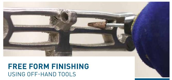
Free form finishing using off-hand tools can provide an excellent finish for metal 3D printed parts. A wide range of abrasive products are available including discs, belts and mounted points which can be used for off-hand or robotic grinding. Ceramic abrasives are recommended for use on stainless steel and superalloys while Silicon Carbide or Zirconia abrasives are best for finishing titanium and aluminium.
