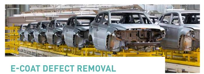
Once the vehicle has been e-coated, baked and sealed, the body goes its first visual check to identify potential defects prior to primer application. Use a Cyclonic or MeshPower disc to remove inclusions and runs. Thanks to the dust extraction features, the discs reduce the airborne dust and risk of contamination. This will assist the operator for the next defect removal process whether manual or robotized.
