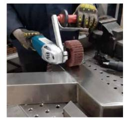
Must be used on a variable speed Right Angle Grinder. Wheels run at lower than normal fixed speeds
