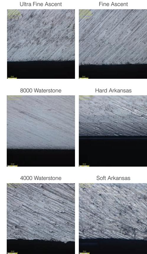
Knife edge comparison under high magnification after final sharpening. Finer grit leaves shallower gouges and a smoother blade edge.
