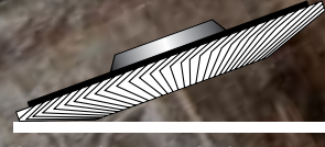
GRIND AT STEEPER ANGLES: 15° – 25°
