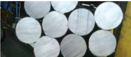
White cut (no burns, cut straightness)
