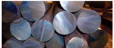
Dark cut (burns, blueing is visible)
