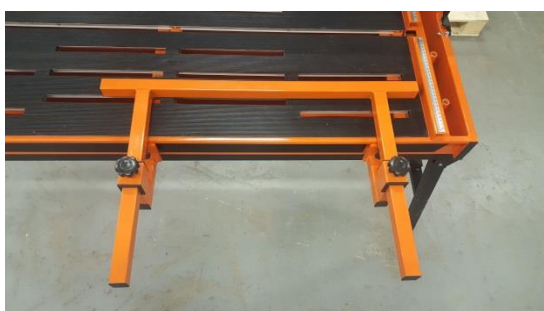
Insert the guide in both supports
