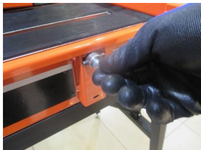
Insert 2 threaded and pinned shafts
