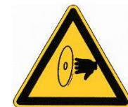
Danger: risk of cut
