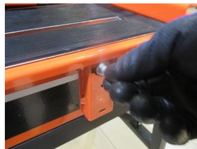
Rotate both shafts by 90°
