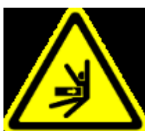
Risk of crushing due to unintentional movement
