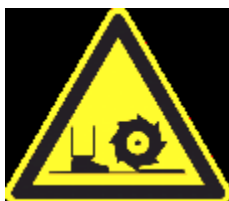
Cutting hazard at the rotating tool
