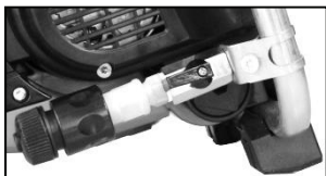
water supply opened (valve lever parallel)
