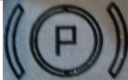
Frein parking desserré
