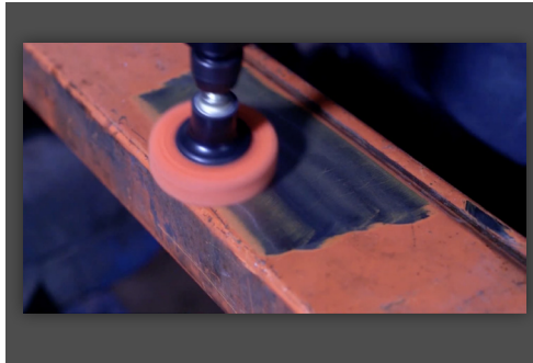
How to remove paint from metal with the Norton Mini Angle Grinder
