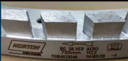
Figure 2 - The engraved arrow in the steel carrier ring
