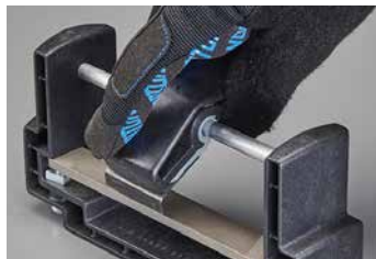
STEP 2 Hold over guide rod at "nose" of tool
