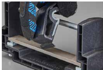
ROUND CORNERS & BLEND WORK After sharpening the blade, glide corners of blade across file (while resting bushing against guide rod) to take off "burr" edges. Keep fingers clear of tool path. This allows for a smoother cut and the ability to blend work.
