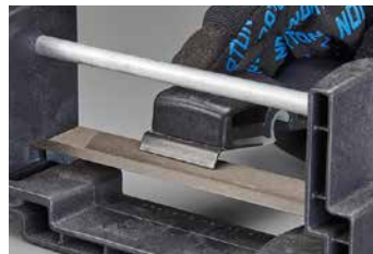
CORRECTING OVER SHARPENED BLADE After blade is initially sharpened, it only takes a few pulls to resharpen again. Additional pulls can cause blade to "fold over" on itself resulting in a dull blade. To correct this move backside of blade across file removing burr edge. Once burr is removed, resharpen.
