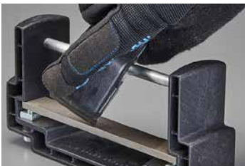
ROUND CORNERS & BLEND WORK After sharpening the blade, glide corners of blade across file (while resting bushing against guide rod) to take off "burr" edges. Keep fingers clear of tool path. This allows for a smoother cut and the ability to blend work.
