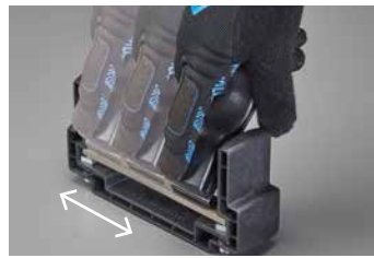
SHARPENING BLADE Bring blade in glancing contact with file as you move it along rod. Do not bear down on file - Let the tool do the work.
